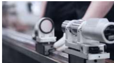
05 STRAIGHTNESS INSPECTION Laser collimator inspection of guide rails.
